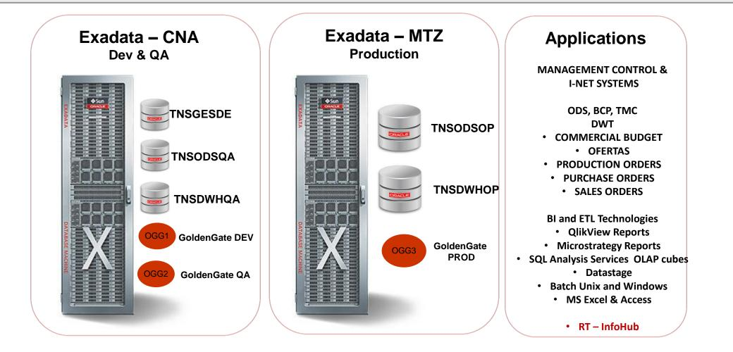
1 Rack – 2 blades DB (28 cores, 512 gigas per blade) - Oracle real application cluster Database Oracle 12C, on Oracle Linux 6.2 3 blades Storage (triple redundancy) with 28 teras
